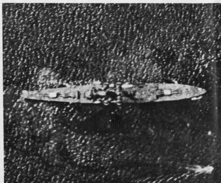
Aerial reconnaissance of Mogami CA shows 3-A-2 battery arrangement. Mogami Class has a Jap raked combined stack, lighter bridge than other Jap CA's. As CL's, these ships mounted fifteen 6-in. guns.
